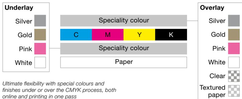
Ultimate flexibility with special colours and finishes under or over the CMYK process, both online and printing in one pass
